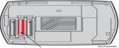
Insert supplied batteries for primary or backup power.
