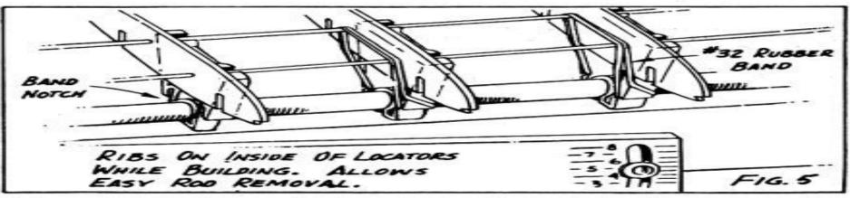
Use a straight-edge over the tops of the ribs to check alignment, also the leading and trailing edge. Now is a good time to see if a rod hole needs reworking. Another way would be to stack the ribs between two rib locators on two rods, then sand uniformly. After all the ribs are fastened down, lay in spars without glue to see that they fit properly without binding, also fit leading and trailing edge. Tip washout can be built into the wing by wedging up the rear rod with balsa wedges.
