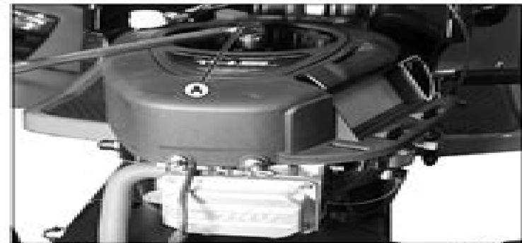
4. Remove the flywheel screen. Use a socket with a breaker bar (A) on the flywheel nut to hold the flywheel in position when performing the test.
