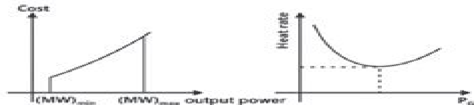
Fig. 3.1 Variation of Cost and Heat Rate with Power
