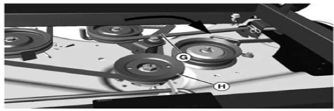
MXML200812031840411-UN: 48 inch mower deck shown. Connect mower drive belt:
