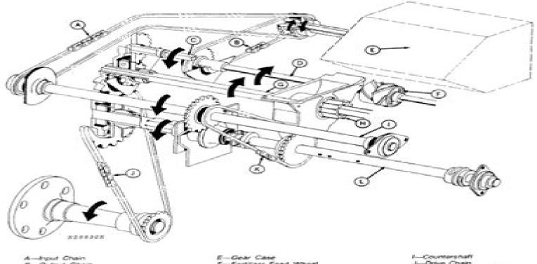
B-Output Chain C-Agitator Shaft D-Fertilizer Feed Shaft
