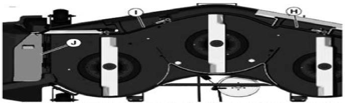
Inspect position of LH baffle (H), center baffle (I), and discharge gate (J). Cycle the linkage to mulch position and back to see if baffles are moving through full range.
