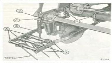
The angle of the teeth may be adjusted at points "A." Spring pressure may be adjusted up or down at "B." Transport clearance is adjusted at "C."
