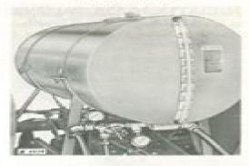
The pre-emergence sprayer attachment is used to apply any liquid chemical form of herbicide in the row at the time of planting.
