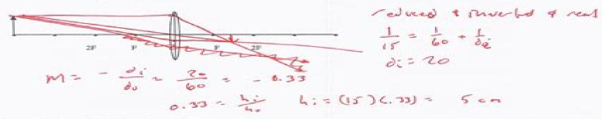
2. A 15.0 cm object is placed 30.0 cm from a convex lens, which has a focal length of 15.0 cm.
