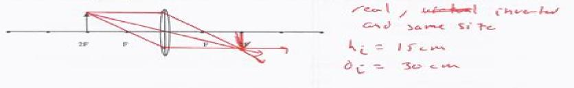
3. A 15.0 cm object is placed 16.0 cm from a convex lens, which has a focal length of 15.0 cm.
