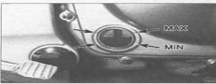
With the engine off, check the oil level in the window located at the lower part of the right crankcase cover. The oil level should be between the Maximum and Minimum level marks on the window.
