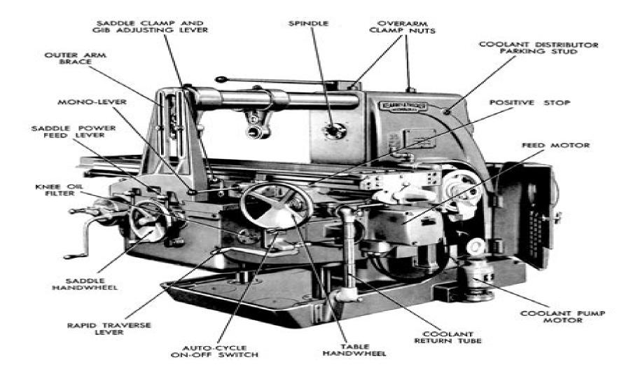
Figure 2. TF Series Plain Milling Machine — Right Front View
