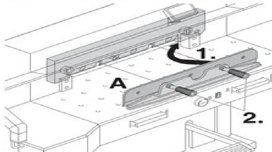
Place the blade to be exchanged with the blade changing tool (A) mounted (1.), into the blade carrier and push it up to the top and screw it into place with the grips (2.).
