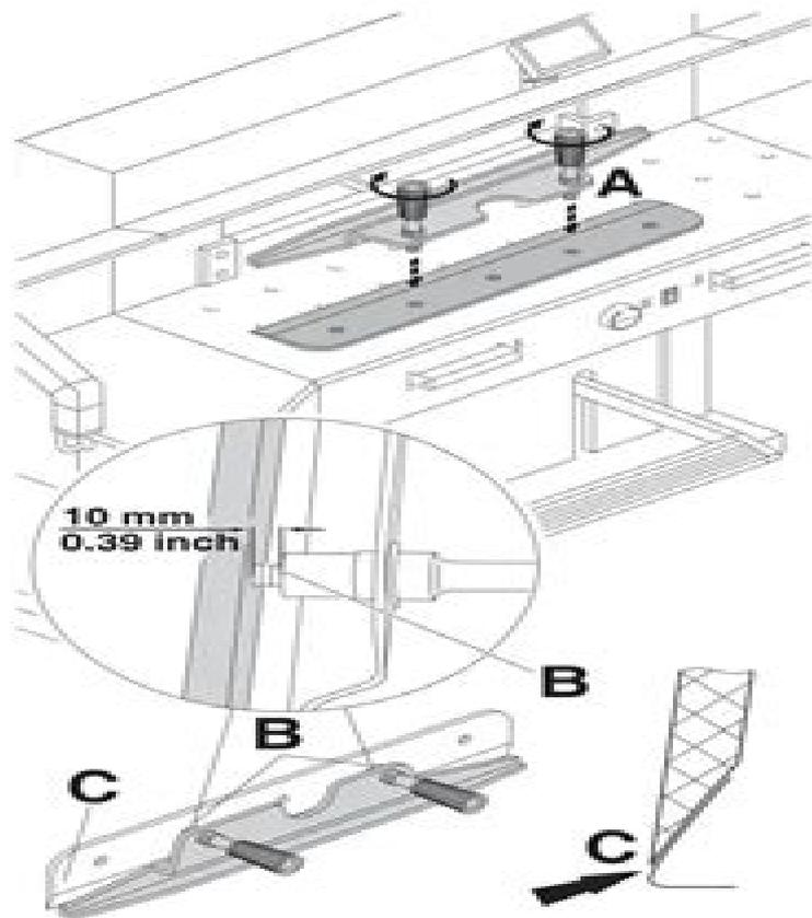
Take the exchange blade carefully out of the blade box and screw it to the blade changing tool (A)
