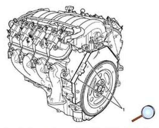
The vehicle identification number (VIN) (1) is located on the left side rear of the engine block and is typically a 9 digit number stamped or laser-etched onto the engine at the vehicle assembly plant.
