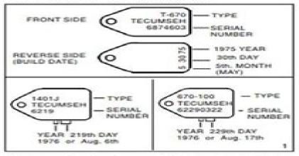
The second method was put in place to standardize 2 cycle and 4 cycle engine identification. The type number has now become the specification number, which is preceded by the engine model as illustrated in Figure 2 and 3.
