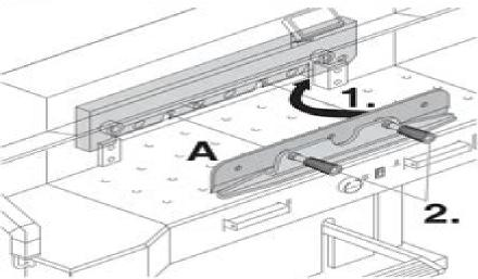
Place the blade to be exchanged with the blade changing tool (A) mounted (1.), into the blade carrier and push it up to the top and screw it into place with the grips (2.).
