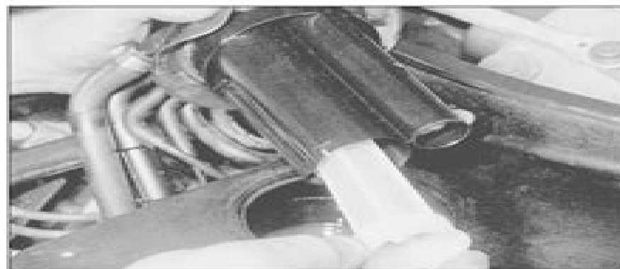
23.4b . . . and twist the round filter to release it
