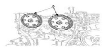
9 Remove the cam shaft.
