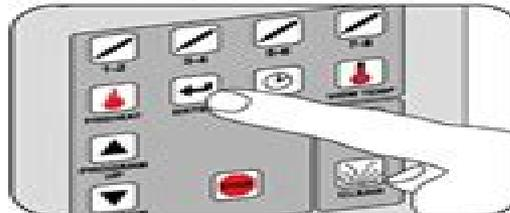
5. Switch the rotisserie on by pulling out the red main ON/OFF switch. Follow instructions on the display and then press "ENTER".
