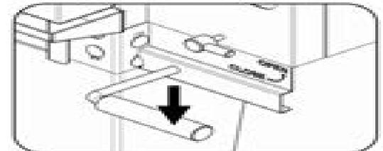
6. Make sure the drain valve (large handle) and the water inlet (small handle) are closed.
