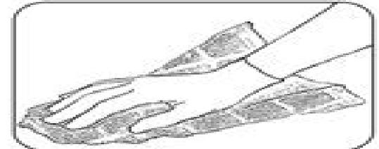
3. Wipe the drip pan clean with a towel removing all particles. **DO NOT PUSH DEBRIS INTO THE DRAINS.**
