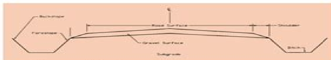
Figure 1: The components of the roadway cross section.
