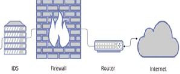
The Intrusion Detection System (IDS) is a powerful security tool for preventing unwanted access to business networks that monitors network traffic for suspicious behavior, analyzes it in advance, and issues warnings when suspicious activity is detected.
