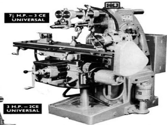
The robust design incorporates conveniently positioned directional controls, independent motor drive to the spindle from a cross-mounted main motor and separate knee motor for feed and rapid traverse, thereby ensuring adequate power, ease and speed of operation with economical and accurate production.
