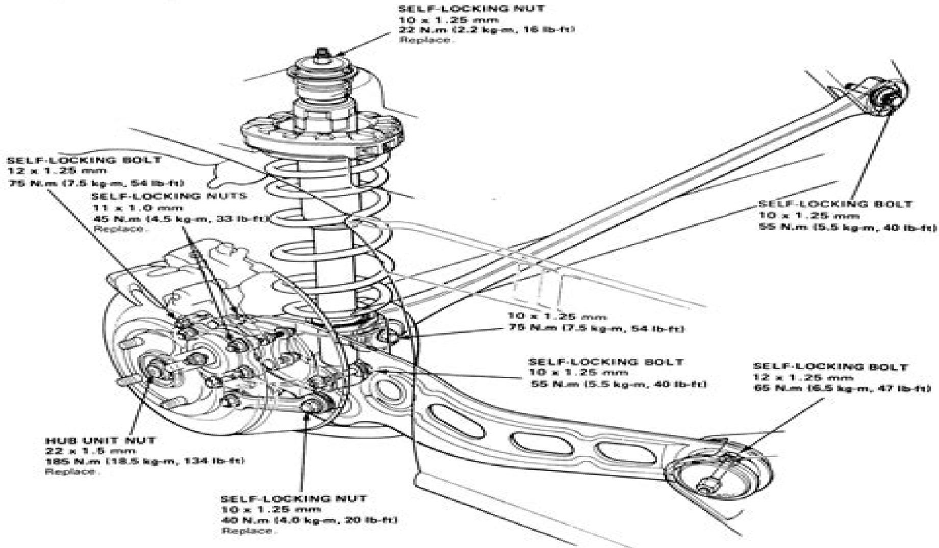
**CAUTION:** Before tightening the bolts and nuts connected to rubber mounts or bushings, the vehicle should be on the ground.
