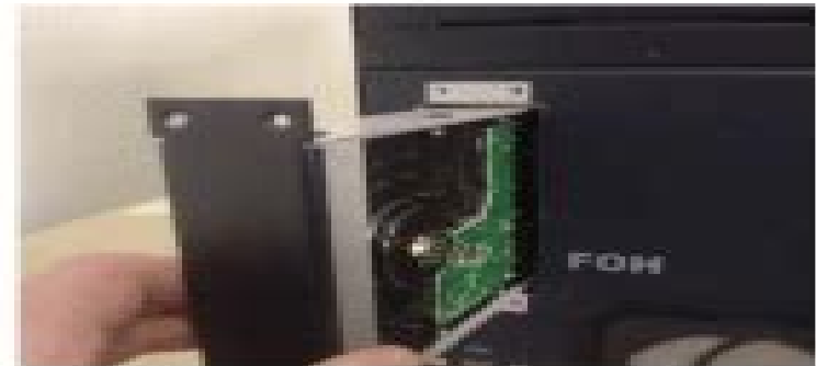
Sliding the hard drive bay from the FOM Rack
