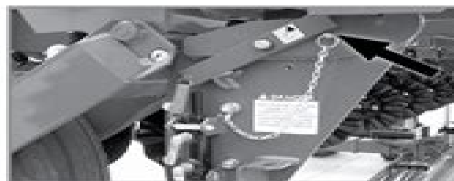
Transport latch locking pin installed
