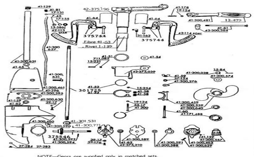
NOTE—Gears are supplied only in matched sets. Part No. 375546. Includes 301531 Pinion Gear and 375187 Prop. Shaft and Gear.
