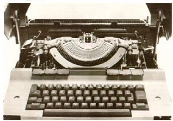
Access to the inside of the typewriter can be achieved after releasing the two cover latches located beneath the machine just in front of the On/Oft Control and Impression Control Lever, Pulling the latches forward will release the cover so that it can be lifted.
