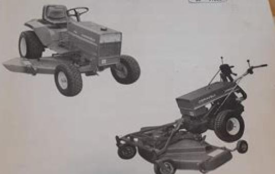
The 40 Inch and the 50 Inch Rotary Mowers are for use with the Gravery 50.00 Series. Tractors and the 8000 Series Tractors. To connect either mower to the 5000 Series. Tractor a front mount kit, part number 15569 is needed.
