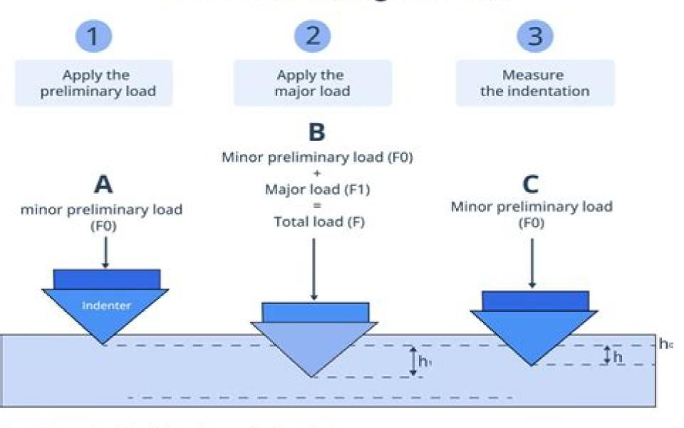
h<sub>0</sub> = Indentation depth by minor preliminary load h = Lasting impression depth
