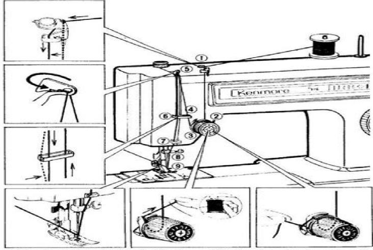
Raise thread take-up lever to its highest position by turning hand wheel toward you. Raise presser foot lever. Place thread spool on spool pin.
