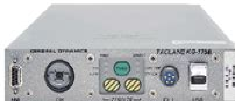
Figure 2.1-2 (U) TACLANE-Mini (KG-175B)
