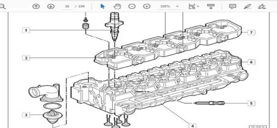
Electro-injector - 2. Electro-injector electric connection terminal - 3. Thermostat valve - 4. Induction manifold - 5. Fuel filling pipe to the injector - 6. Cylinder head - 7. Chassis bracket for injectors electric outfit - 8. Electric connector - 9. Electroinjector wiring harness - 10. Cotters, cup and spring.
