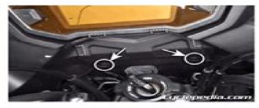
Remove the bulb maintenance lid. Depress the center pin on the two trip clips (circled). Pull the lid downwards and out to release the four retaining tabs.
