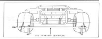
Align the toe-in gauge with the marks on the tires as shown. Check the readings on the gauges scales.
