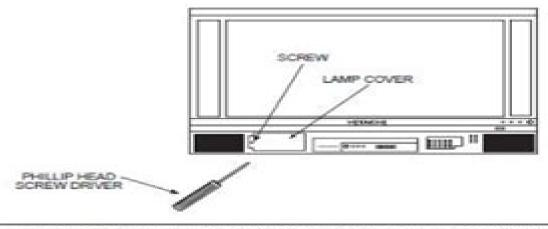
NOTE: THE LAMP IS VERY HOT AND MAY CAUSE FIRE OR SEVERE BURNS. WAIT AT LEAST 30-45 MINUTES TO ALLOW THE LAMP TO COOL BEFORE PROCEEDING WITH LAMP REMOVAL.
