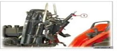
Once the separation has finished, remove the steering column (1) by lifting it up slowly with a hoist.
