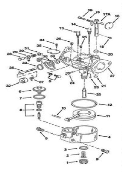
DISASSEMBLY: Use exploded view as a guide. The numerical sequence may generally be followed to disassemble unit far enough to permit cleaning and inspection. Note: On some models, it is necessary to first move throttle lever (17A) from shaft before throttle valve (16) can be removed. Main nozzle (22) can be removed by inserting a small tapered puller and lightly tapping out of housing.
